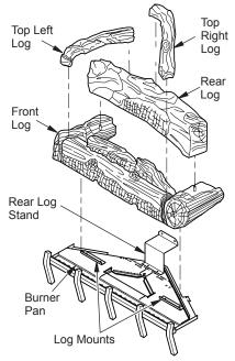
Figure 46 - Installing Logs
